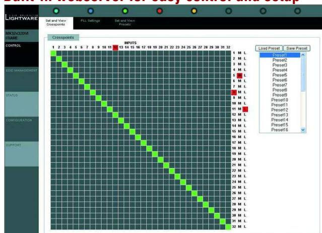
Controls all functions of the router like IP configuration, routing, EDID Management, system status monitoring, Color space and color range control, audio sample rate conversion, etc.
