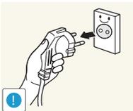
Hold the plug when disconnecting the power cord from the power socket.
