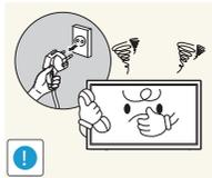
If the product generates abnormal sounds, a burning smell or smoke, disconnect the power cord immediately and contact Samsung Customer Service Centre.
