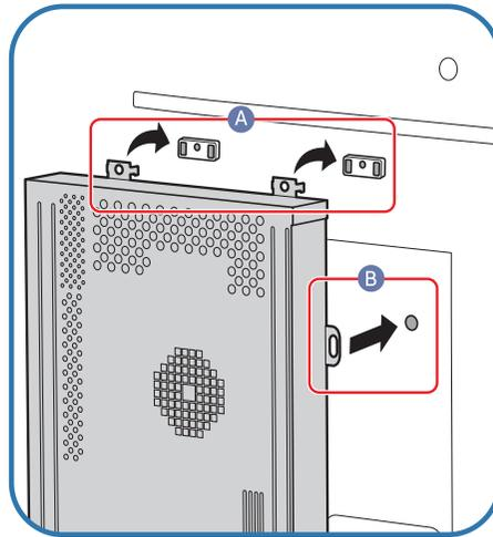
2 First insert the tabs of the network box into the slots marked (A) on the attachment frame. The tabs should hook onto the frame. Then, align the holes marked (B).
