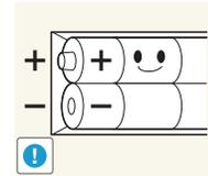
When replacing the battery, insert it with the right polarity (+, -).
