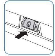
Use the remote control within 7 m to 10 m from the sensor on the product at an angle of 30° from the left and right.
