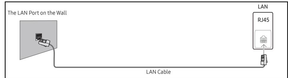
If you have a Dynamic Network, you should use an ADSL modem or router that supports the Dynamic Host Configuration Protocol (DHCP). Modems and routers that support DHCP automatically provide the IP address, subnet mask, gateway, and DNS values your product needs to access the Internet so you do not have to enter them manually. Most home networks are Dynamic Networks.
