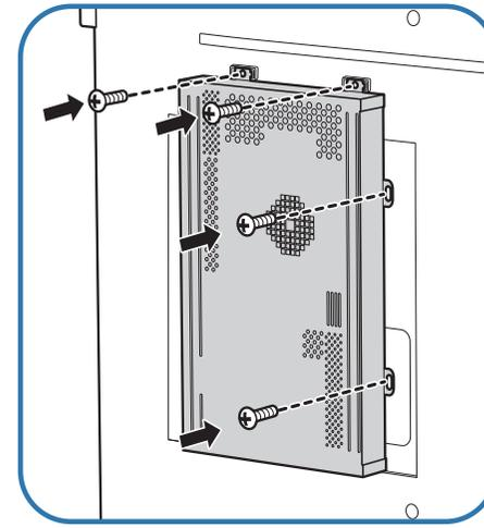
3 Attach the network box to the fixed attachment frames.
