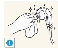
Clean any dust around the pins of the power plug or the power socket with a dry cloth.
