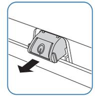
To use remote/eco sensor, make sure the sliding panel key is protruding from the bottom of the product.
