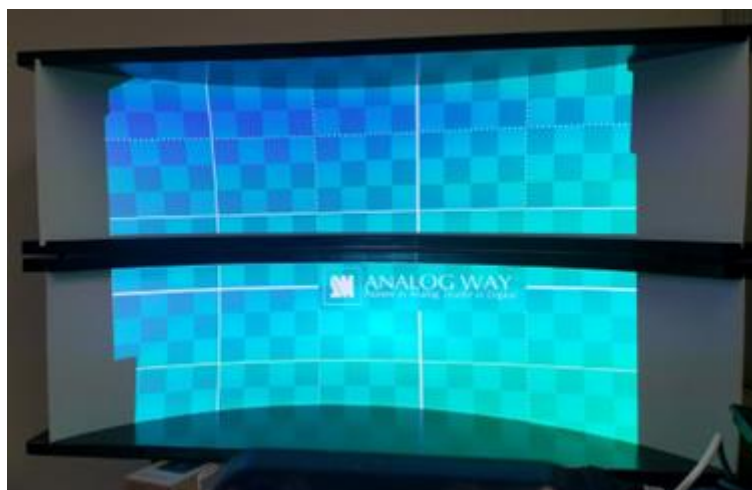
Fig. 79 - Autocalibration: The projection test image after the initial calibration
