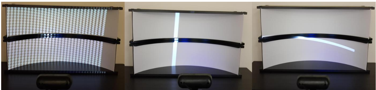
Fig. 77 - Autocalibration: scanning and calibrating the projection surface
