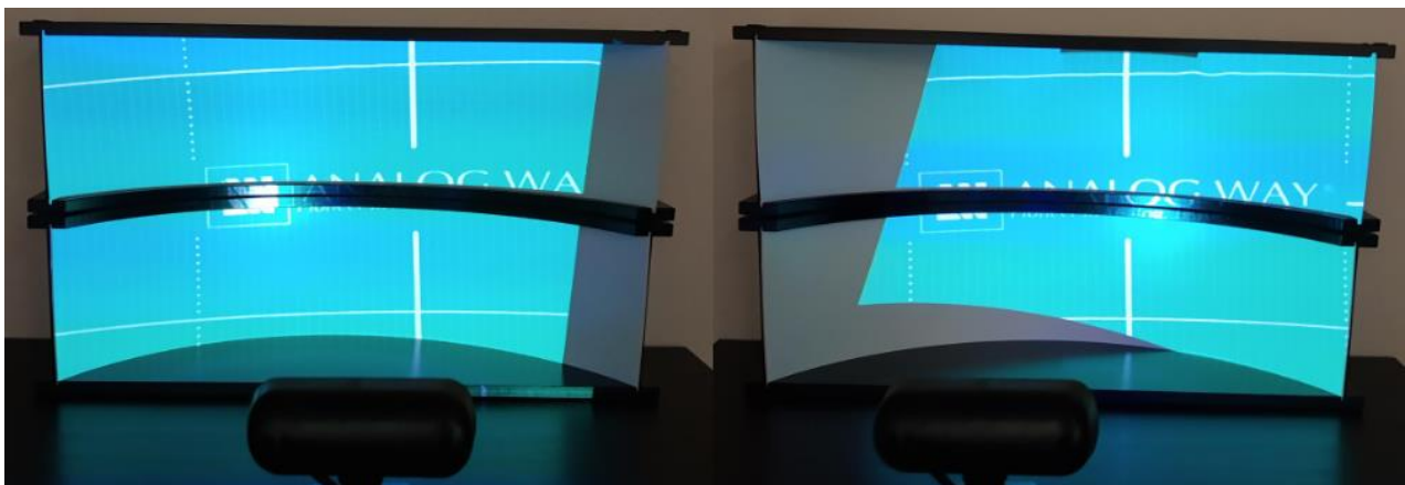
Fig. 78 - Autocalibration: test images after the initial calibration process (2 projectors)
