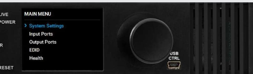
Easy setting and menu navigation are assured by the color graphic display and the comfortable jog dial control: keep dial and click while getting accurate feedback, well visible in various lighting conditions.
